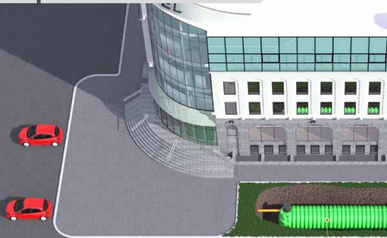
UNDERGROUND RAINWATER TANK
